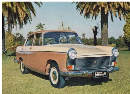
A publicity photo of the Freeway. The horizontal lines of the grille were an attempt to visually widen the car.
